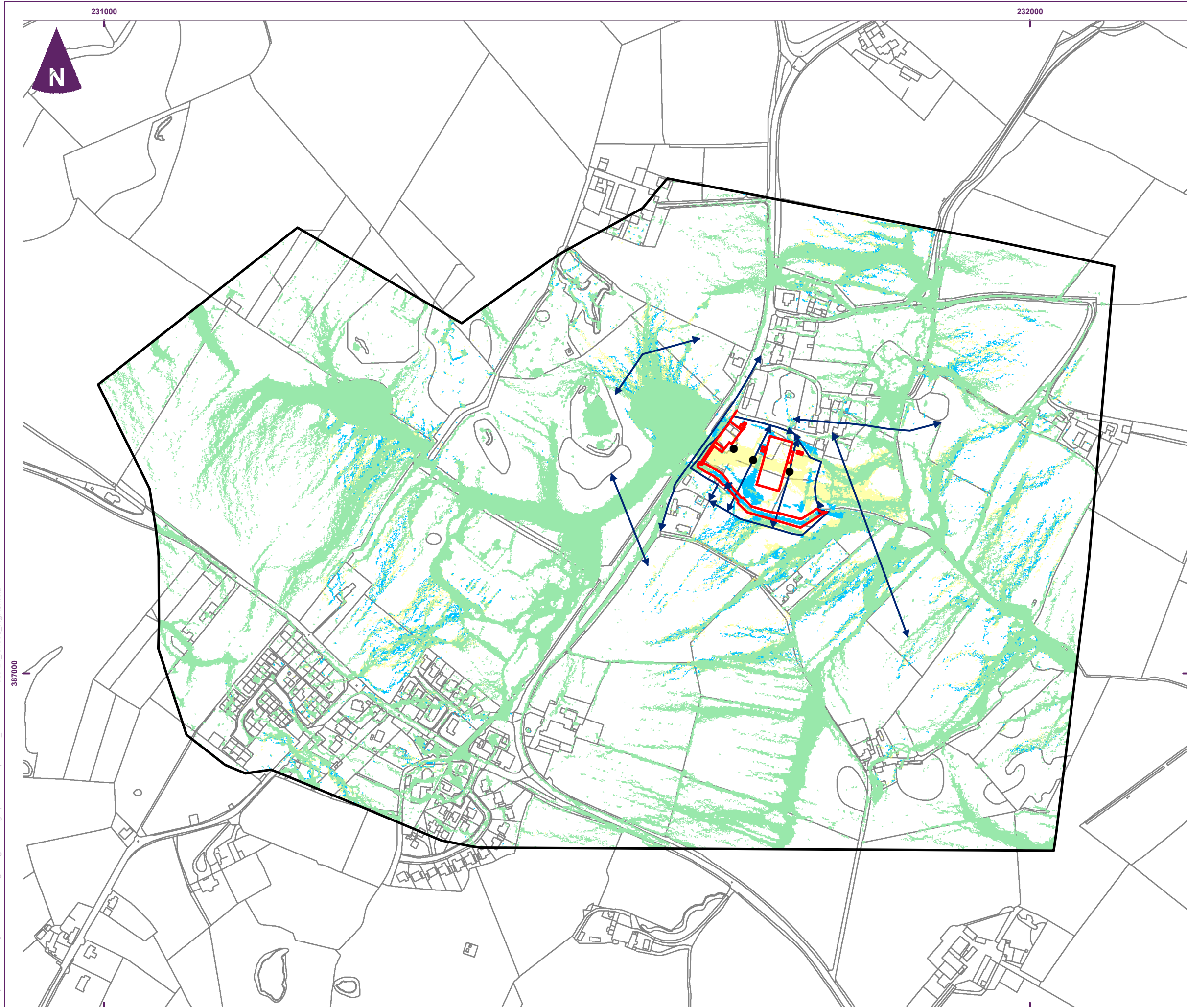
Figure 7.9 Llanfaethlu peak pluvial flood extent difference 1:100 year AEP (1 hour storm event) plus climate change (20%)
