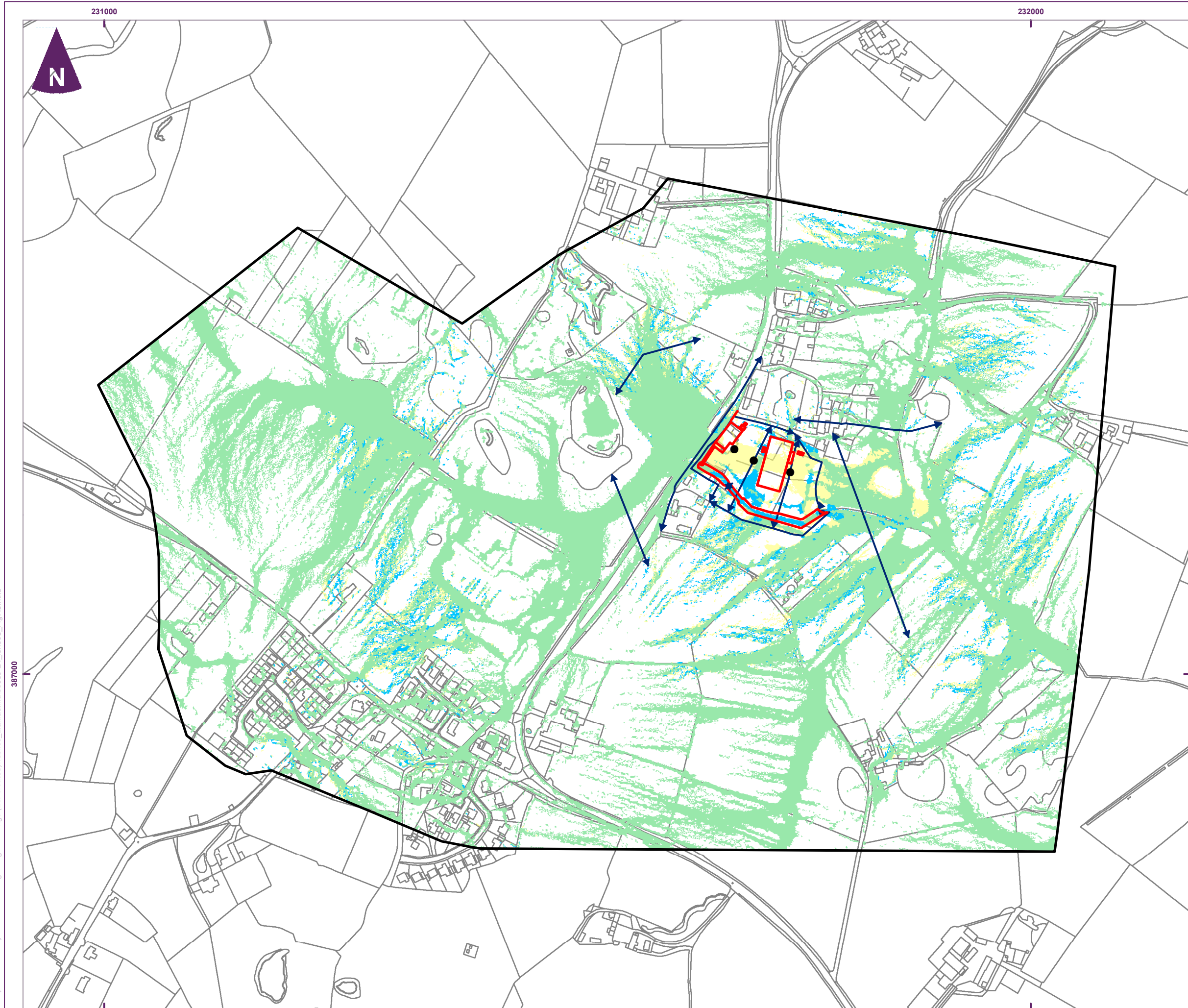
Figure 7.8 Llanfaethlu peak pluvial flood extent difference 1:1000 year AEP present day (1 hour storm event)
