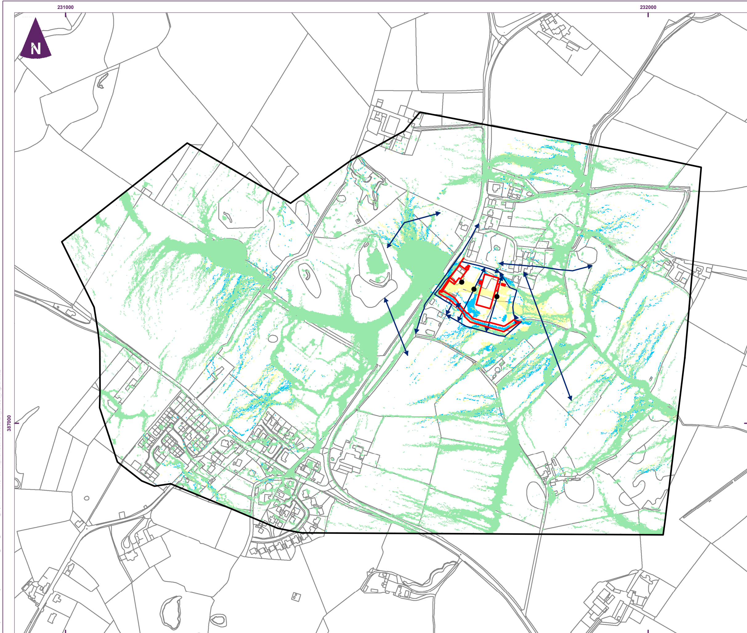
Figure 7.7 Llanfaethlu peak pluvial flood extent difference 1:100 year AEP present day (1 hour storm event)
